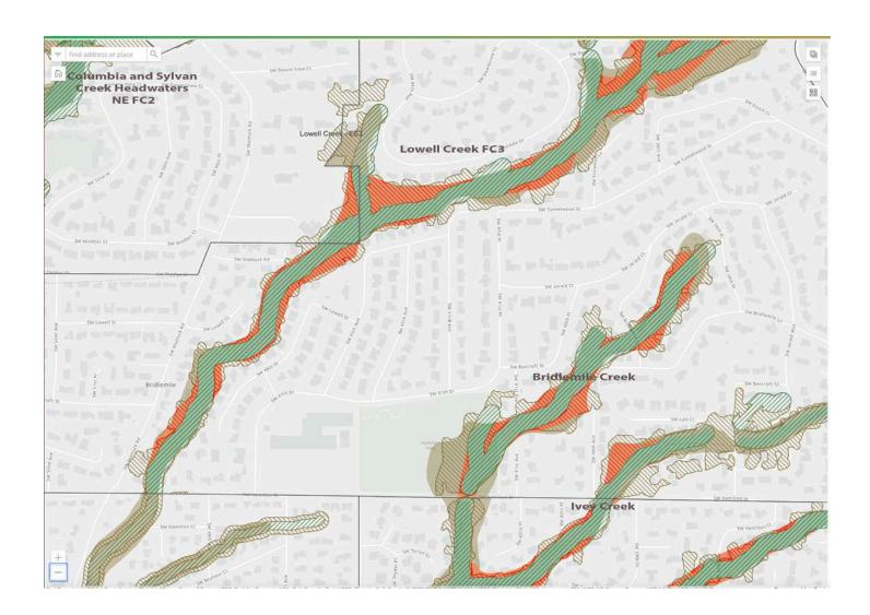
Protection zone "P" is the highest zone for protection Conservation zone "C" opens up for possible construction
