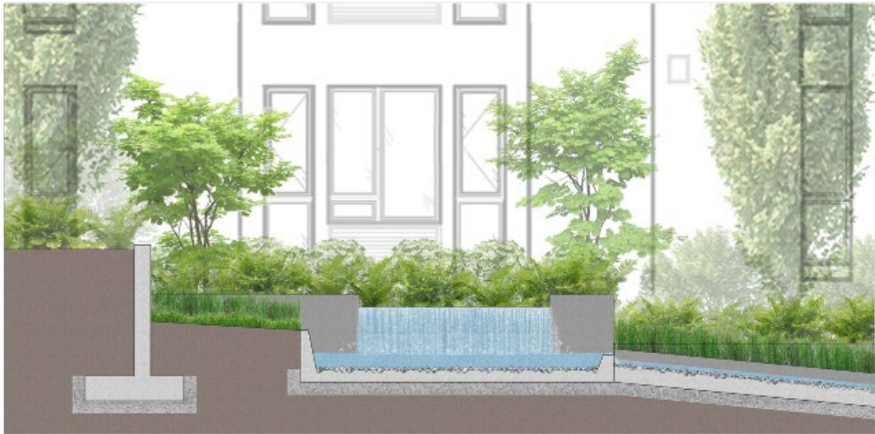
WATER FEATURE SECTION B - B
