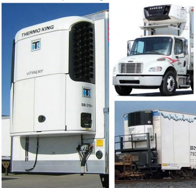
Figure 11: TRUs on Trucks, Trailers, and Rail Cars 42
