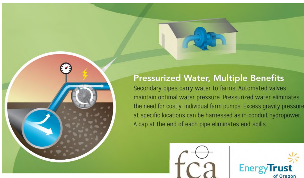
Figure 2: Energy Trust of Oregon and Farmers Conservation Alliance Illustrate Irrigation Modernization Option for In-Conduit Hydropower
