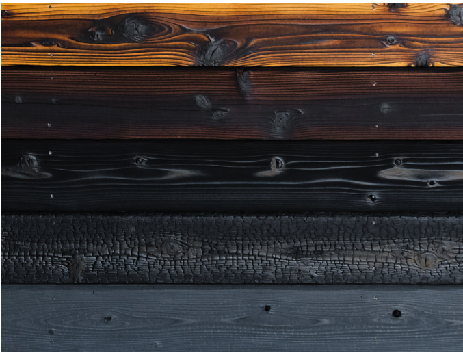
Carbonized Wood at Building Entry
