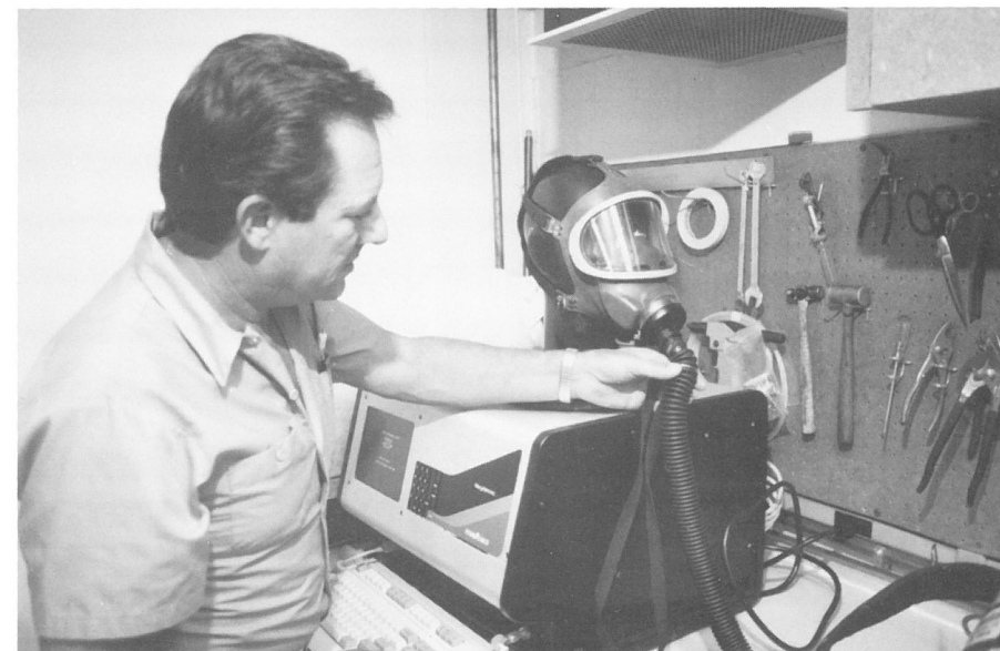
The latest technology in SCBA functions, the POSI-CHECK for testing for proper flow and status of the regulator
