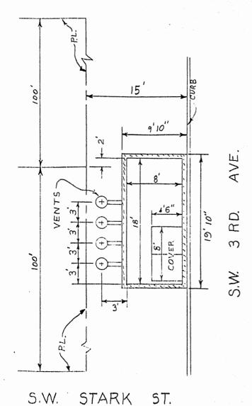
SCALE NONE DRAWN BY LLB CHECKED BY H+4 1/4 SEC, 3029 PRE-CAST VAULT STD. NO. 818 LA-10 WITH A 4'-6"X 8' SIDEWALK DOOR AND 4-1'-10" DIA. VENT CASTINGS
