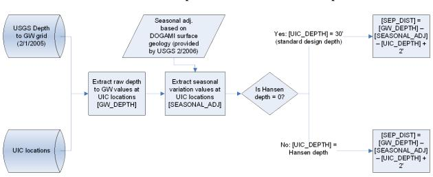
Figure 4-1 Process Used to Calculate Separation Distance at Each Sump Location
