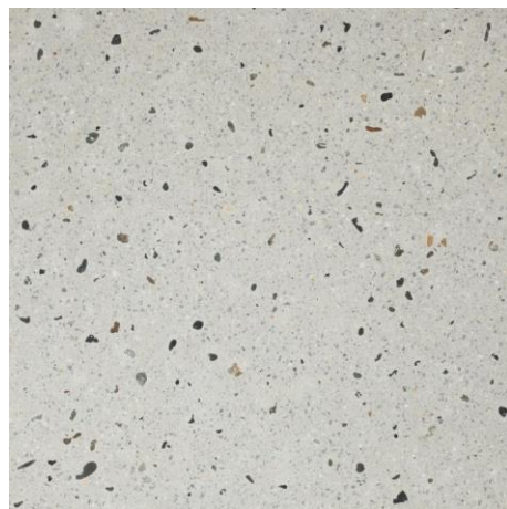
PRECAST CONCRETE BASE WALL WITH SLATE HONE FINISH
