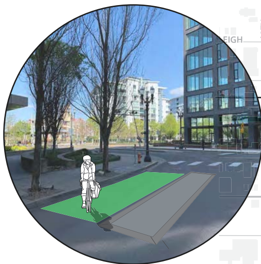
Traffic diverter redirects westbound vehicles and provides a connection for people biking.
