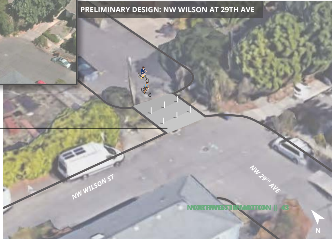
A path through the diverter allows an easier connection for people biking
