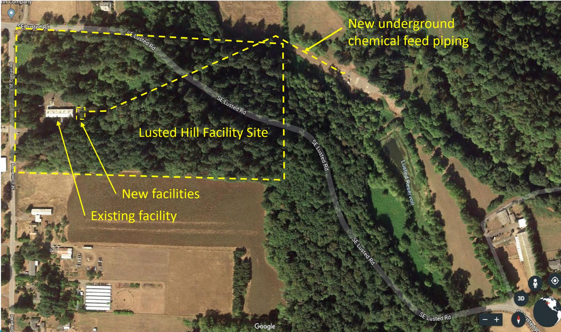
The improved corrosion control treatment facility will be located alongside the existing facility
