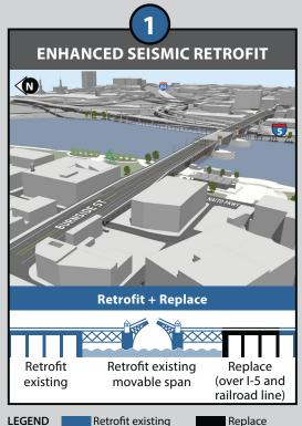
Upgrade of the existing bridge to meet current seismic standards. This includes a combination of retrofitting portions of the bridge and replacing others.
