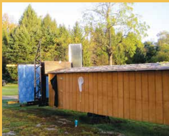
The tunnel: an apparatus for safely testing effectiveness of materials and designs for deterring bird collisions. Photo by Christine Sheppard, ABC
