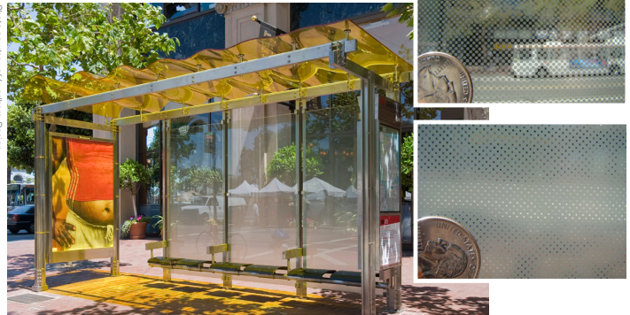
ABOVE: The City's new bus shelters designed by Lundberg Design use a subtle frit pattern to indicate the barrier. This design, called "SF Fog," is effective in alerting both people and birds to the glass. INSETS show how the frit pattern is more dense at the bottom and dissipates like the City's fog at the top.
