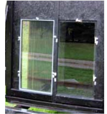
A panel of fritted glass, ready for testing. Photo: Christine Sheppard, ABC
