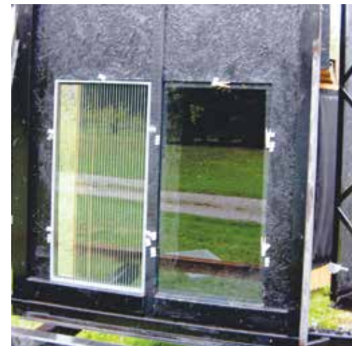
Glass panes are being tested at the Powdermill Tunnel, as seen from the outside. Photo by Christine Sheppard, ABC
