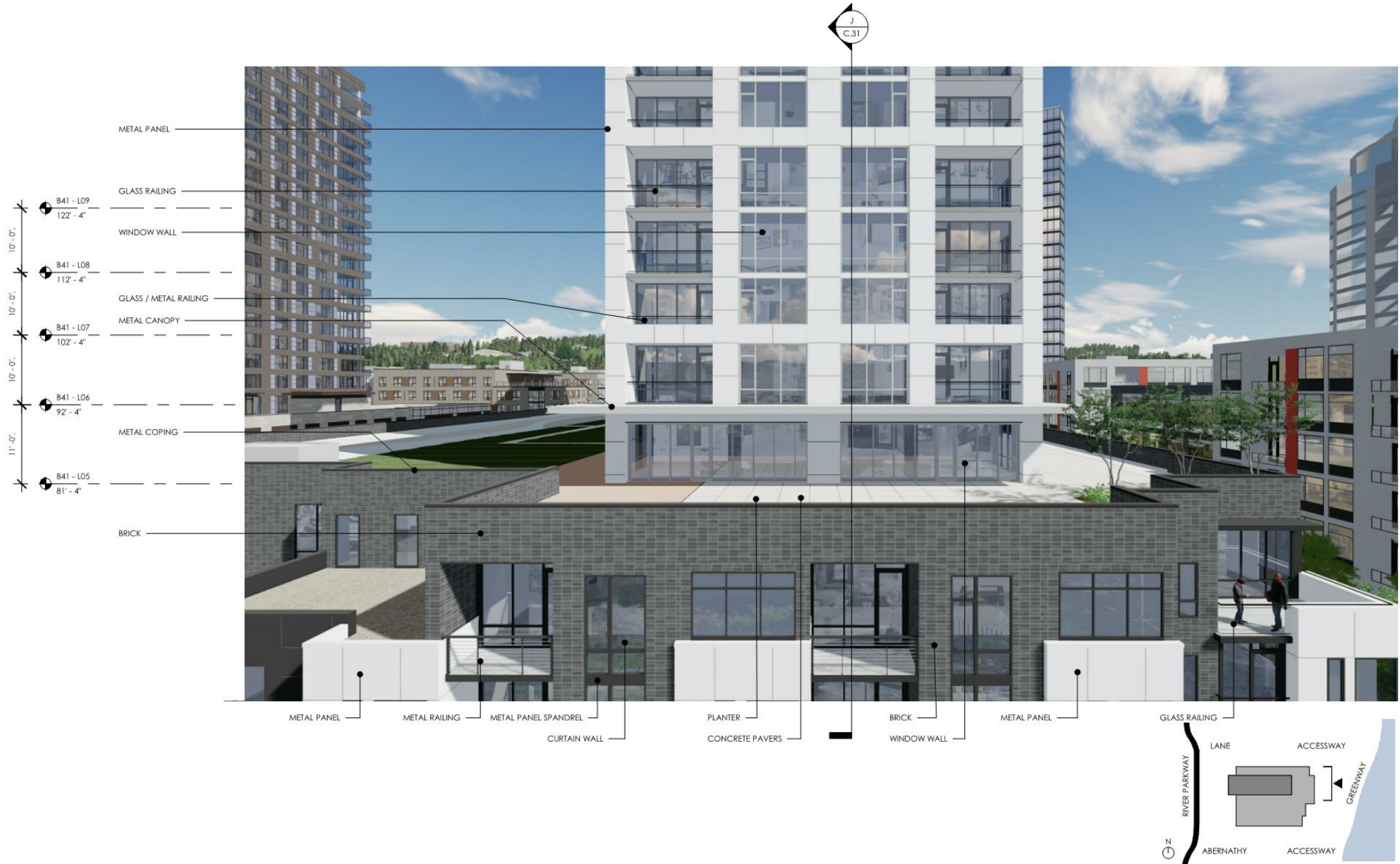
BLOCK 41 - ENLARGED ELEVATION LEVEL 5 AMENITY
