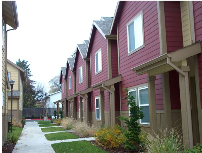
Amendments to the pedestrian standards will allow entrance pathways accessing up to four units to be as narrow as three-feet wide, even on a large site with more than 20 units.
