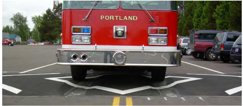
Speed cushions support effective emergency response while slowing passenger vehicles and enhancing neighborhood livability and safety.
