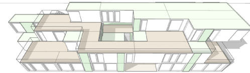
Container Blocks - Original 20' small blocks are reconfigured into larger sizes for efficiency.
