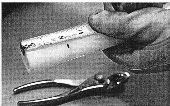
Figure 6-16: Measure 2" of tubing
