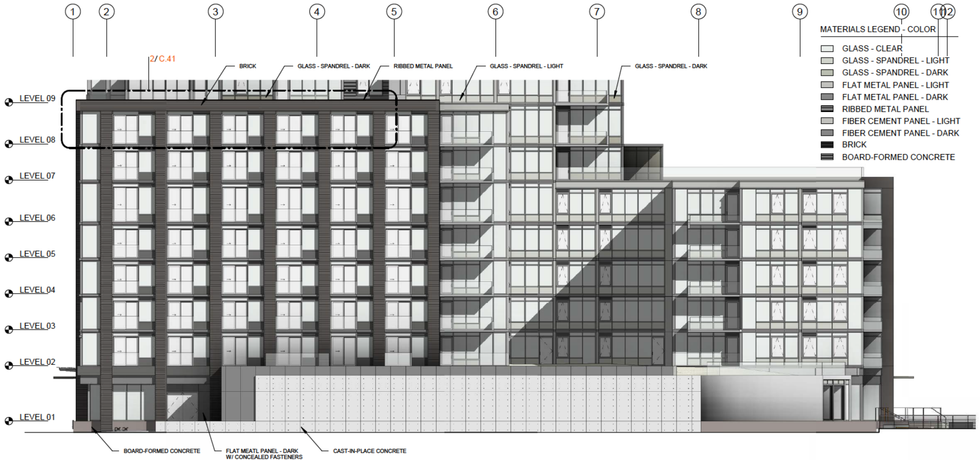
① STREET-LEVEL ELEVATION - SOUTH 1/16" = 1'-0"
