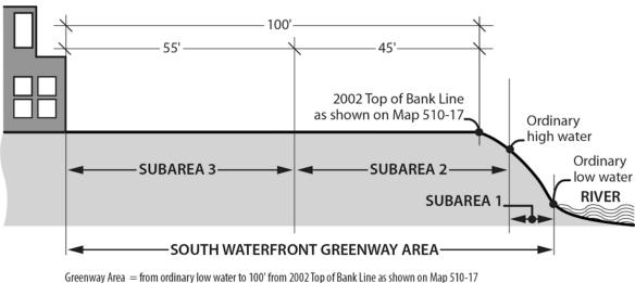
DELETE <del>Figure 510-2</del> South Waterfront Greenway Area and Subareas REPLACE with Figure 510-3 below
