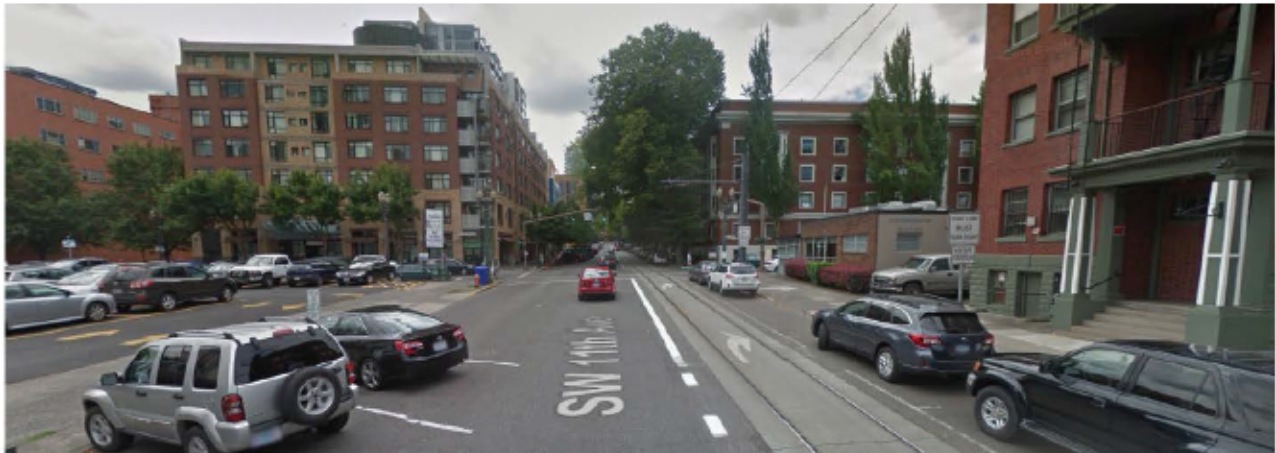
Exhibit 2. Example of Enhanced Transit: Southbound Business Access and Transit (BAT) lane on SW 11th Avenue from SW Stark Street to SW Clay Street, shared with Portland Streetcar alignment. This is an example of how Enhanced Transit treatments can benefit both buses and streetcars.
