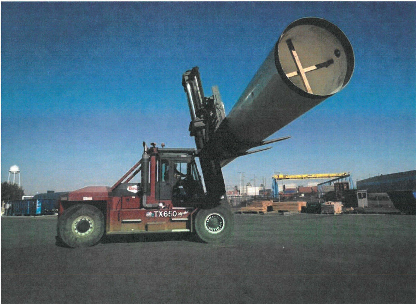
PORTLAND TRIBUNE: JAIME VALDEZ - A large forklift carries a pipe from one Northwest Pipe Company building to another, to be finished before being trucked to a project site. The 2X4s in the pipe prevent it from flexing too much.
