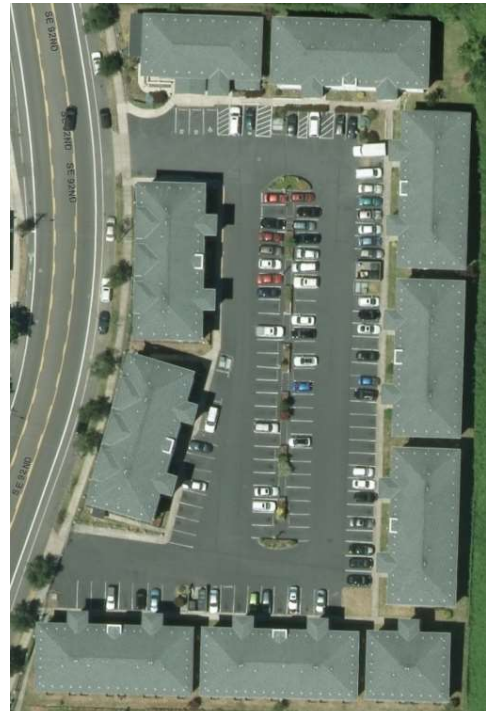
Apartment development in East Portland providing parking at the current required ratio of one space for each unit, leaving little room for outdoor areas and trees.
