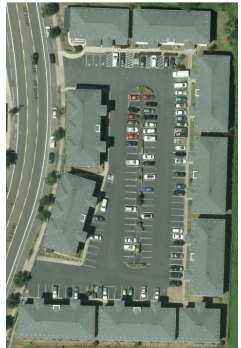
Apartment development in East Portland providing parking at the current required ratio of one space for each unit, resulting in 37 percent of the site paved for parking.
