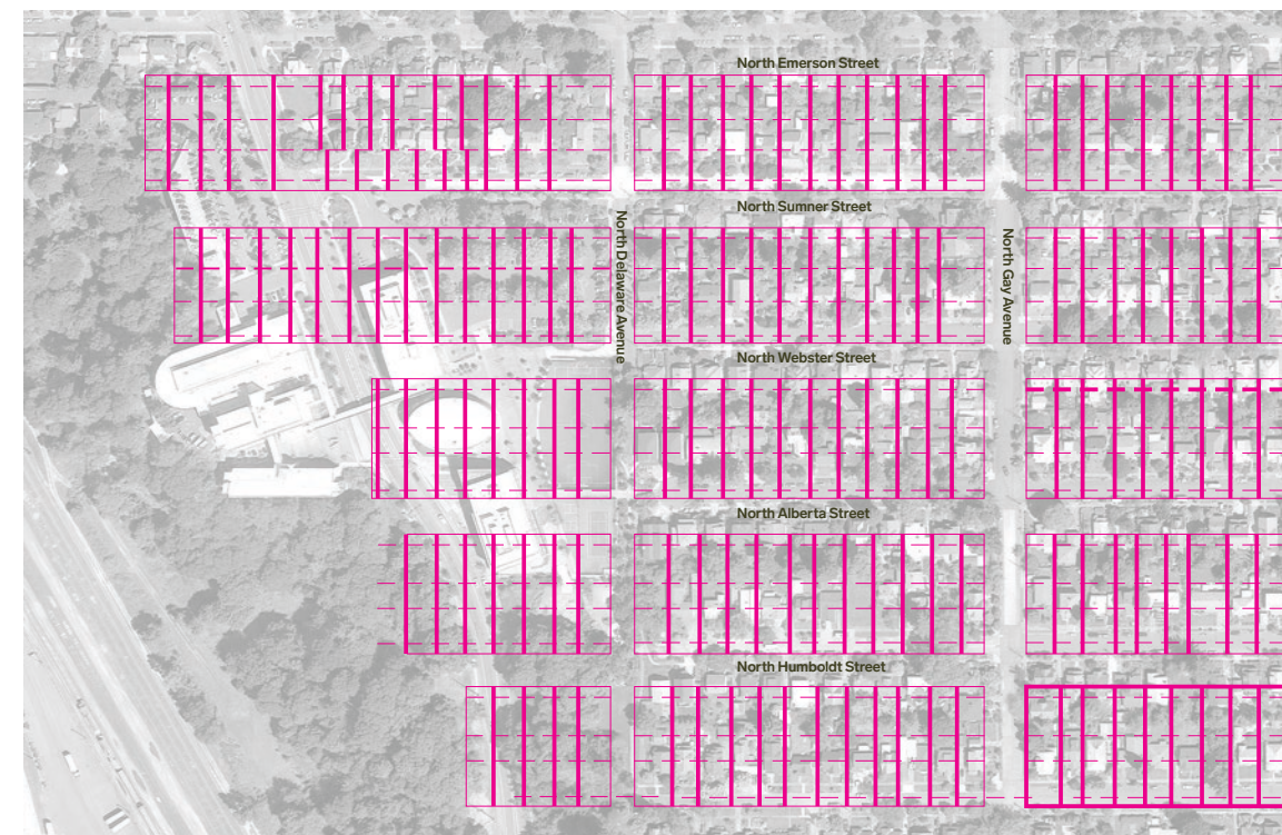
Block analysis shows fine-grained frontage onto longer east-west streets like Sumner and longer side yards along the shorter north-south avenues like Delaware
