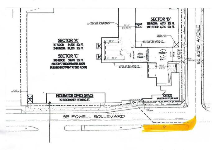
The east-bound turn lane from Powell is only 50 ft. long and may not be sufficient length for larger vehicles including moving trucks and passenger vehicles with trailers.
