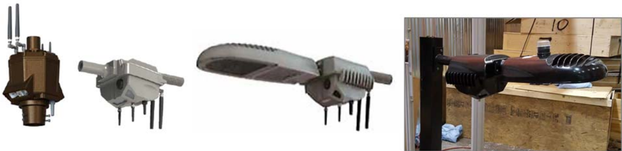
Images of AT&T/GE/intel sensor nodes and sensor nodes attached to LED street lights.
