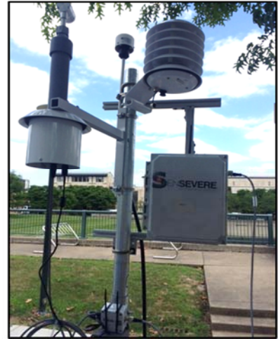
Images of three air quality sensor devices. From left to right, Argonne National Laboratory/University of Chicago's Array of Things Node, Apis' SensorCell Node, and SenSevere's RAMP device.
