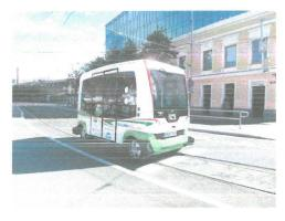
The little low-speed EZ 10 pictured is in use in projects around the world. While only 13 feet long, or about the same as a subcompact, its electric propulsion system enables the passenger compartment to extend the entire length of the vehicle, giving it a capacity for 12
