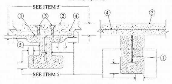
1. Steel Supports — W8x28 steel beam min size or steel joists 10K1 or 16K2 min size with a max tensile stress of 30,000 psi or 12K3 or 12K5 min size with a max tensile stress of 24,000 psi.
