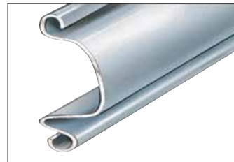
No. 4 – Curved-faced single crown slat available in up to 16-gauge steel, up to 18-gauge stainless steel, or up to 14-gauge B&S aluminum. Depth of crown: 7/8", 25/8" on centers.
