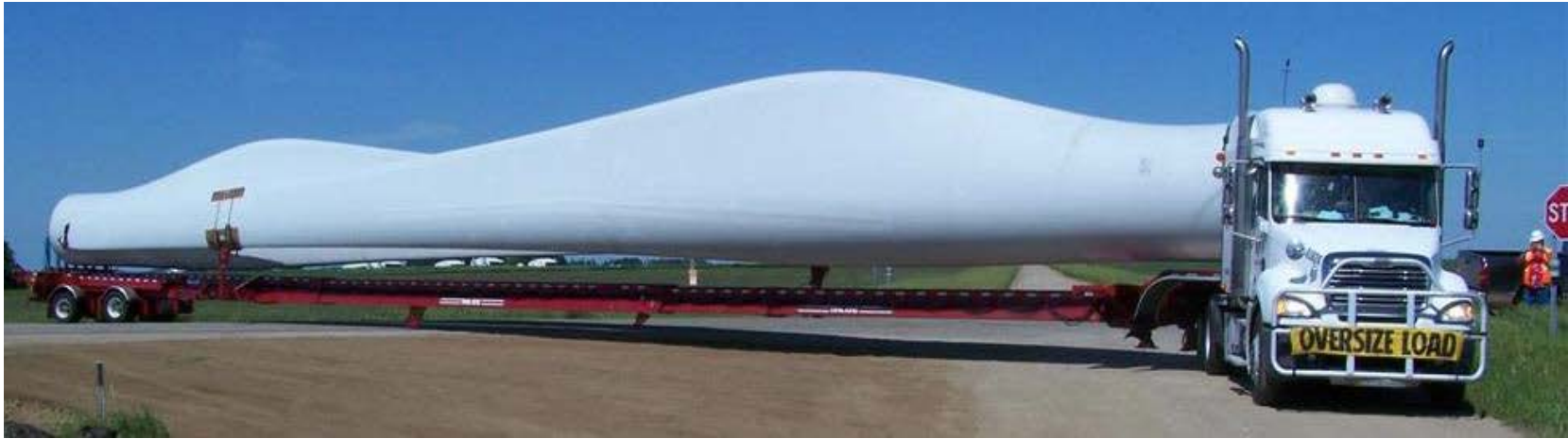
WIND TURBINE BLADES ARE SPECIALIZED OVER-DIMENSIONAL LOADS
