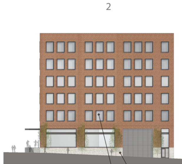
Optimize daylighting and utilize the advantages of current technology with larger window punches in the brick veneer
