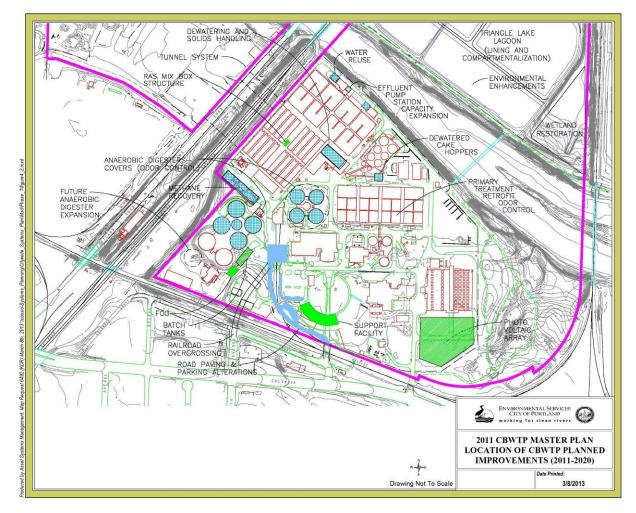
Figure 6.10 Columbia Boulevard Wastewater Treatment Plant Master Plan
