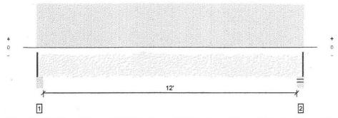
All locations are measured from the outside face of left support (or left cantilever end). All dimensions are horizontal.; Drawing is Conceptual
