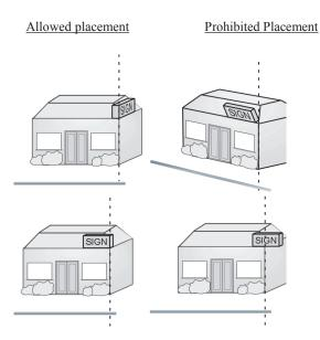
Figure 14 Pitched roof sign placement
