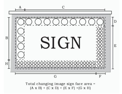
Figure 8 Measuring Changing Image Sign Features Created by Projected Light
