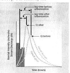
**Figure 7.** A comparison of hydrographs before and after urbanization. The discharge curve is higher and steeper for urban streams than for natural
