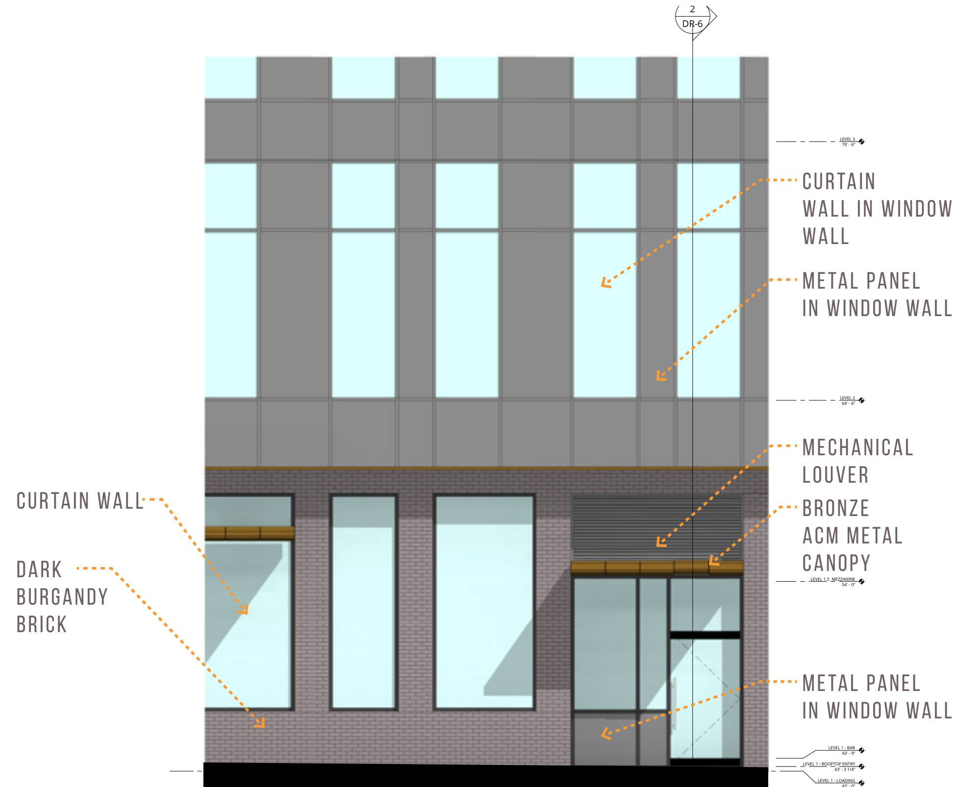
ENLARGED ELEVATION - ROOFTOP BAR ENTRANCE
