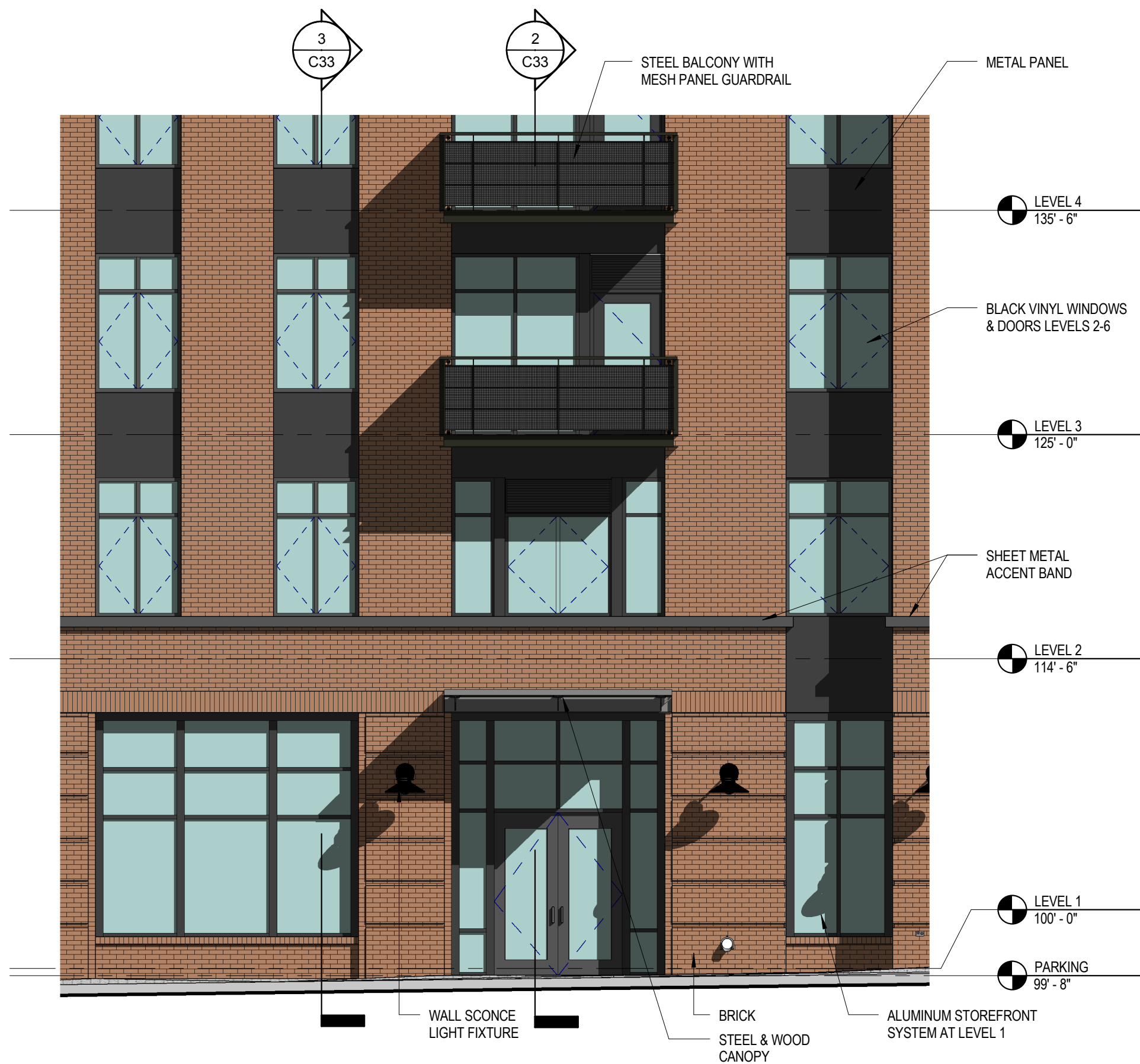
ENLARGED WEST ELEVATION ① 3/16" = 1'-0"
