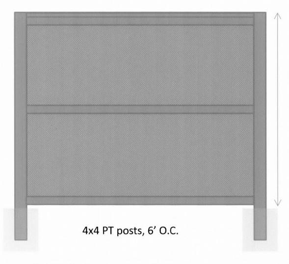
Three 2x4 PT rails and top cap, set at 6", 40", and top of fence. 6" cedar fence boards set close together, for privacy.
