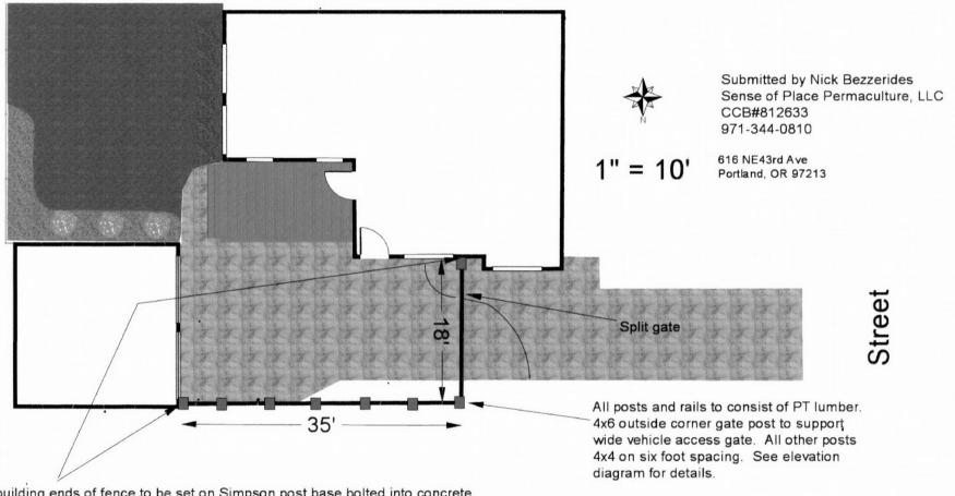
Posts at building ends of fence to be set on Simpson post base bolted into concrete. Post also lag bolted to building. Top of post flashed to direct water away from building.
