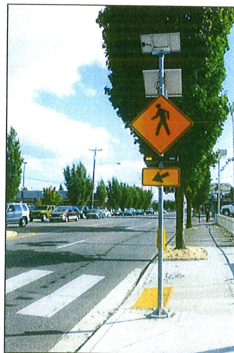
Rapid Flash Beacons get drivers' attention with blinking yellow lights attached to a pedestrian crossing sign. Pedestrians push a button to turn on the lights before crossing the road.
