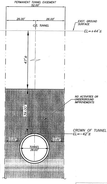
VERTICAL ELEVATIONS SHOWN ARE BASED ON CITY OF PORTLAND VERTICAL DATUM (CPD). CPD IS U.S. GEOLOGICAL SURVEY DATUM (NGVD) PLUS 1.375 FEET.
