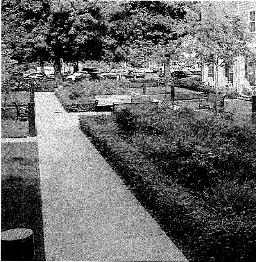
This is a view of the courtyard at the Buckman Terrace Apartment complex. The courtyard's planted areas have been designed to function as stormwater retention facilities. In addition, (and typical of most courtyards) the courtyard offers visual and physical relief for the residents of the building.
