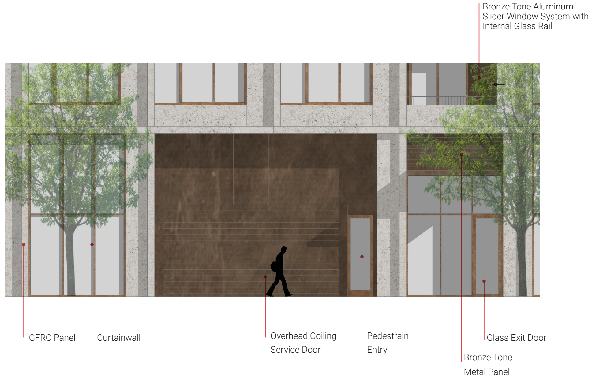
South Elevation @ Service Entrance
