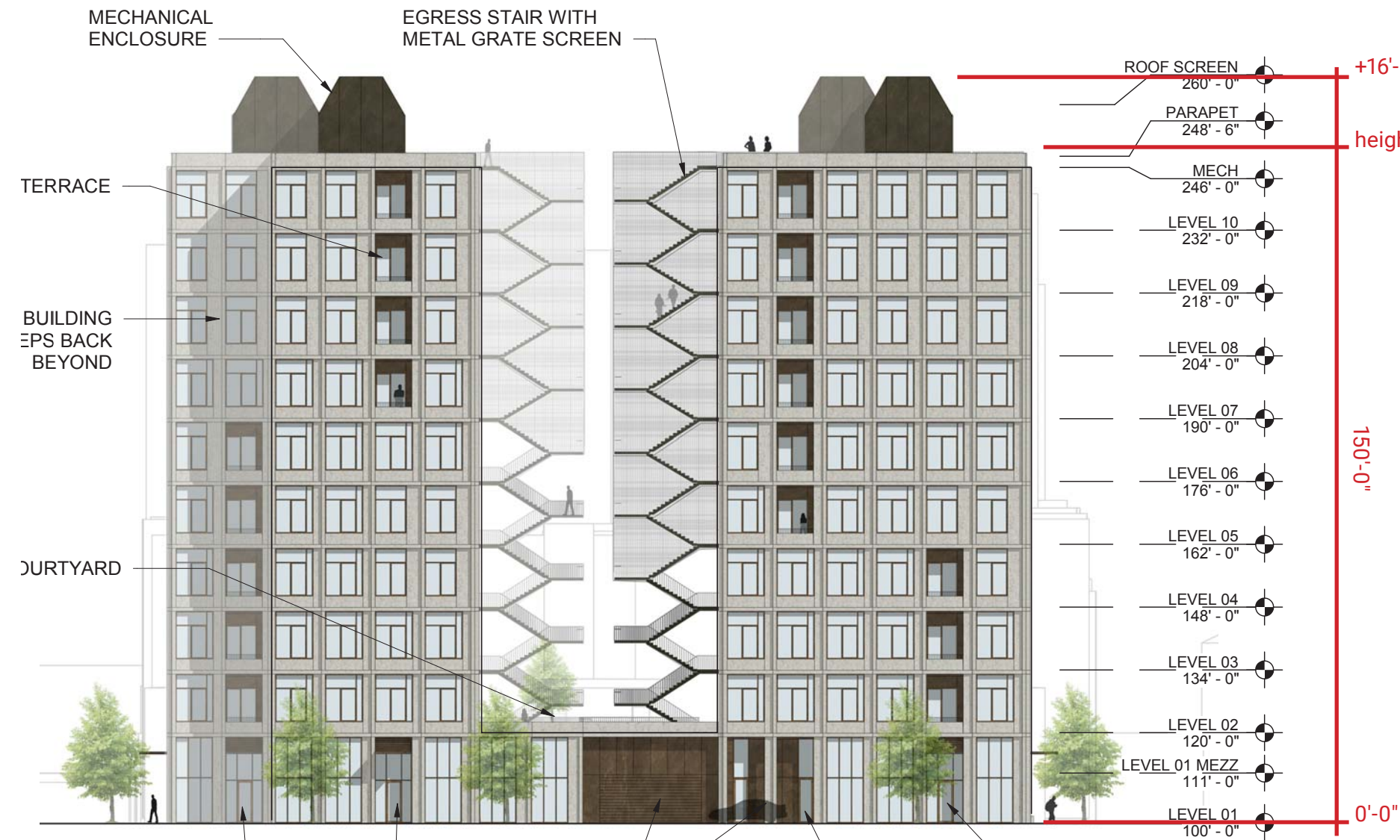
WEST ELEVATION ALONG 14TH
