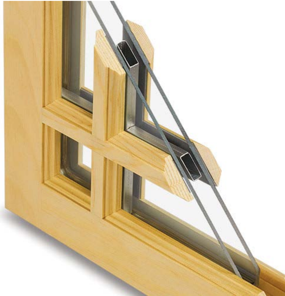
Simulated Divided Lites with Interior and Exterior Muntins and Spacer Bar
