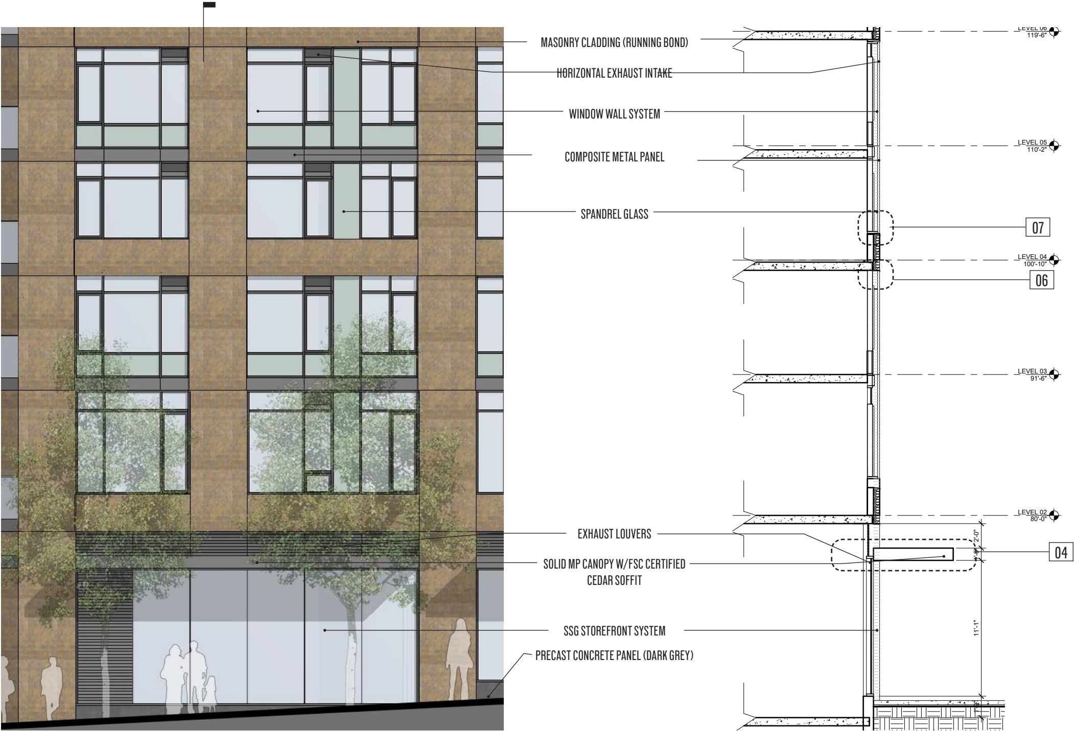
WALL SECTION @ WEST FACADE -TYPICAL TOWER
